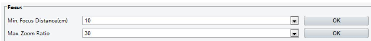
2. Under **Focus**, configure **Min. Focus Distance** (unit: cm) and **Max. Zoom Ratio**.
